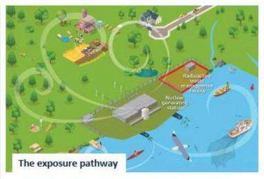
This figure illustrates a conceptual model of the environment around a generic nuclear generating station site (including a generic radioactive waste management facility) to show the relationship between releases (airborne emissions or waterborne effluent) and human and ecological receptors or exposure pathways.
